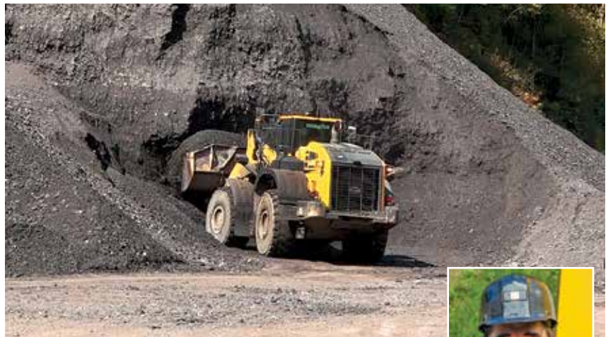
Operator Elbert Addair appreciates the AJSS on the Komatsu WA500 wheel loader because it increases visibility. "They're pretty smooth and operator-friendly," said Addair. "I like the way the 500 is set up so you can clean your windows better on the front. We get good service out of them."
