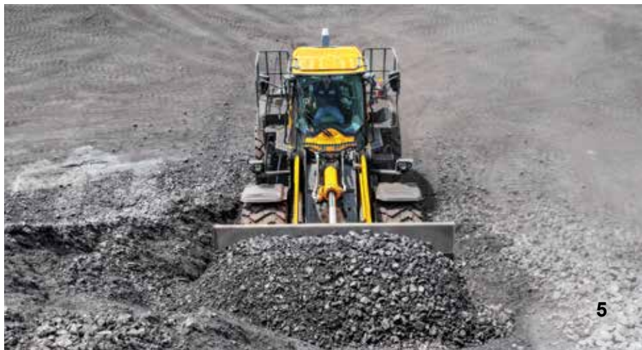
An operator moves coal with a Komatsu WA475 wheel loader.
